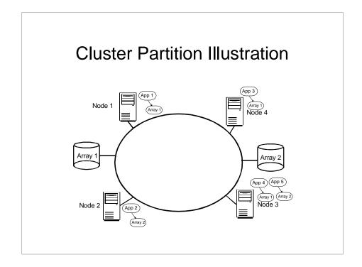
Five applications active on four nodes. Each application is attached either to array 1 or to array 2.
