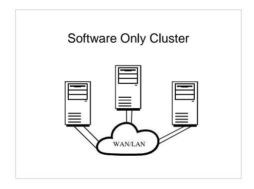
Typical configuration of a software only cluster: Individual nodes connected by a network, using replicators to mirror the individual disc devices. This (by design) looks exactly like just a bunch of computers connected to a net, except that they have connection redundancy.
